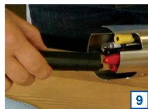
**10** Carefully screw the electrode into the sensor using the electrode key (E-532-TOOL) until hand tight.
