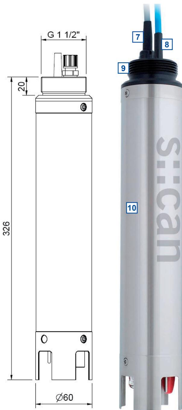
Dimensions of ammo::lyser / fluor::lyser in mm
