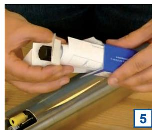
**6** The pH- and reference electrodes are protected with a cap. Before removing the cap cut the cable strap that fixes the cap.
