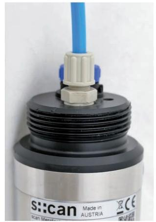
The connection to the cleaning valve depends on the used type of cleaning valve.
