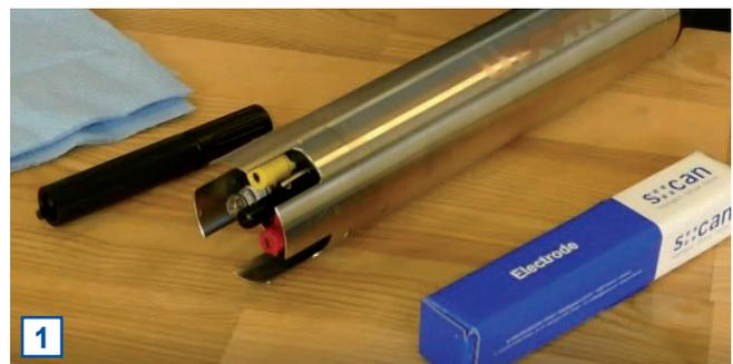
**2** Clean the sensor as explained in section 9.1. Finally dry the electrodes and electrode head with an absorbant paper tissue.
