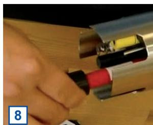
**9** Putting a thin film of vasiline onto the O-ring makes it easier to screw in the electrode.
