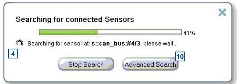
**5** When the automatic search procedure is finished, all connected probes and sensors will be displayed. Those sensors that are connected for the first time and not installed will have the Status *Found new sensor*. These sensors are listed as *New Sensors* below also.
