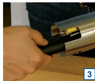
**4** Remove the old electrode from the slot and check if there is any dirt or moisture within the electrode slot. Whipe it clean and dry with a paper tissue if needed.
